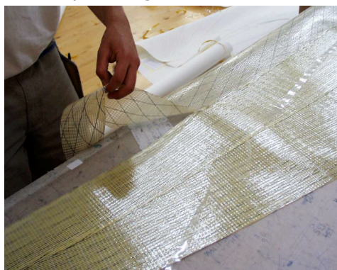
Picture No. 16: Step 2: Remove the plastic film as you are putting the panels together
