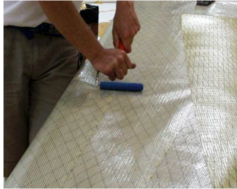
Picture No.18: Step 4: Use a roller over the taped joint to prevent air pockets and to affix the tape to the surfaces.
