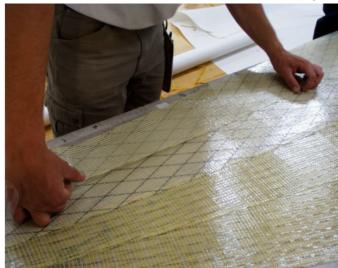
Picture No.15: Step 1: Place the second panel over the taped panel, and let them intersect over the seam allowance area.
