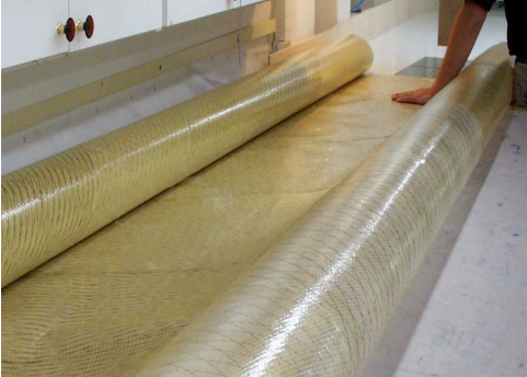
Picture No.22: The sail is rolled along the joints for easier activation
